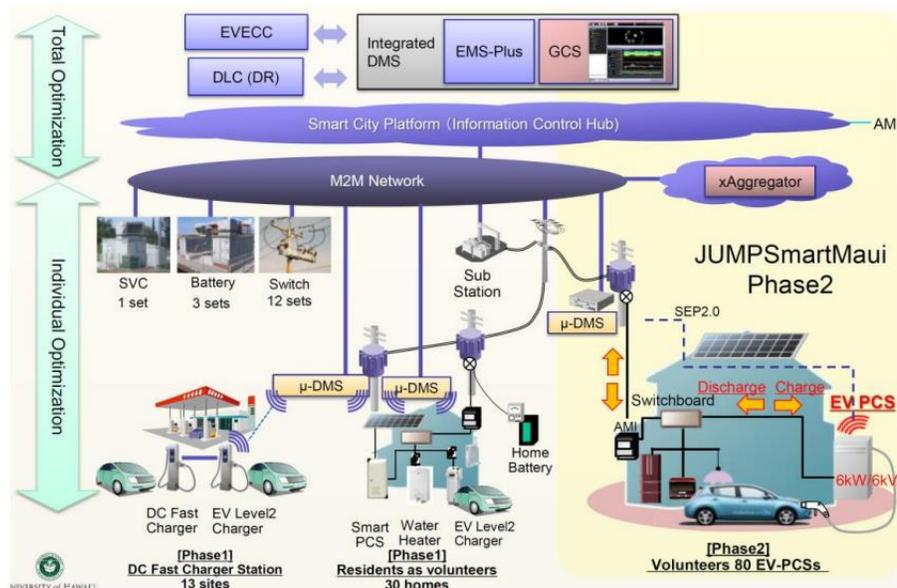
Figure 3 Overall structure of JUMPSmartMaui Smart Community System
