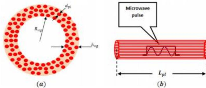
**Figure 1.** (a) Beam pattern and filament distribution after propagation and (b) schematic diagram of a cylindrical microwave waveguide formed by plasma filaments.
