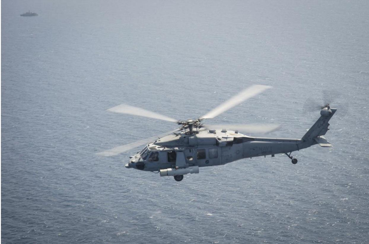
An MH-60S Sea Hawk helicopter from the "LASERHAWKS" of Helicopter Sea Combat Squadron (HSC) 26, Detachment 2, equipped with the Airborne Laser Mine Detection System (ALMDS) conducts flight operations on August 4th, 2014. US Navy photo.
